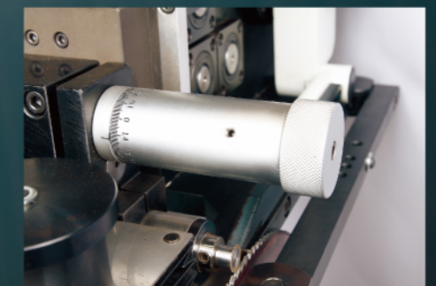
Grinding wheel left and right adjusting button 砂輪左右調整鈕
