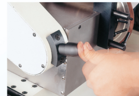
Locking Device for Grinding Wheel Dismantling 拆卸砂輪的剎車裝置
